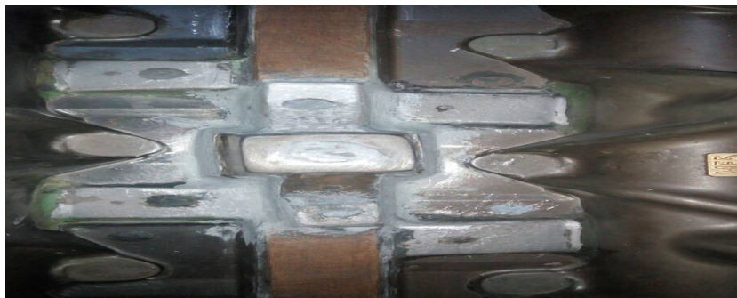
Figure 9: Previous gate shape
