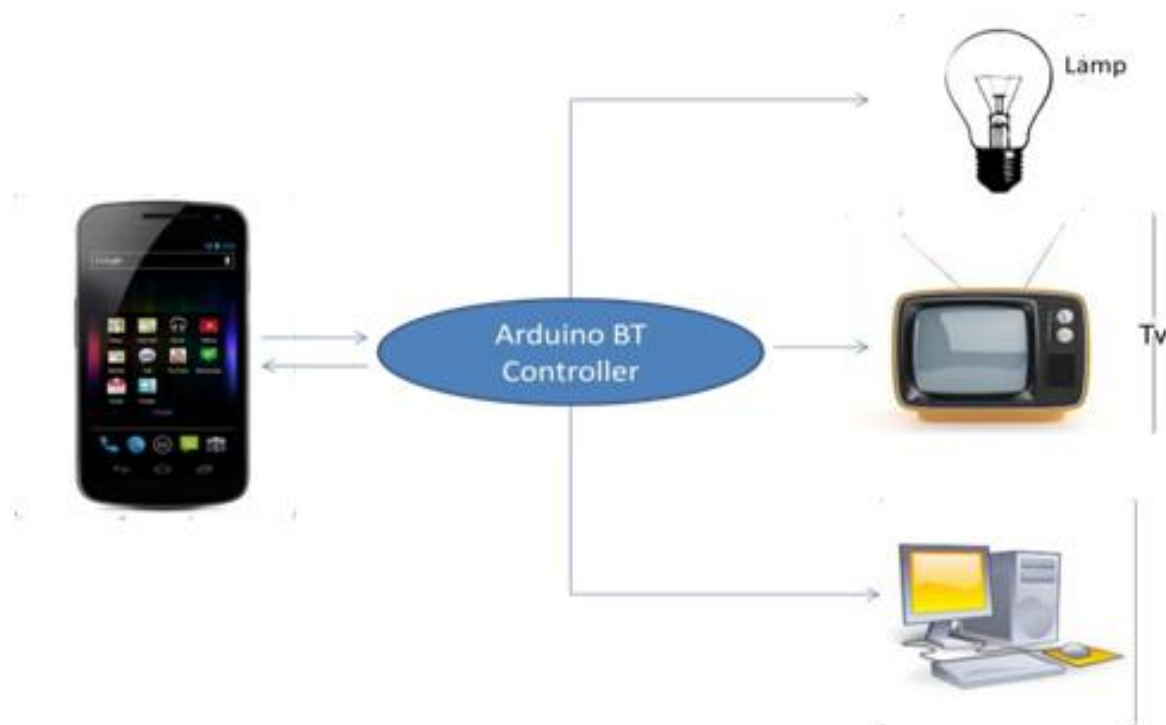
Fig. 2:Block diagram of Home Automation
