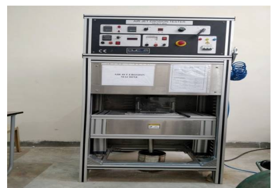
Fig 3.2 Air Jet Erosion Test Machine
