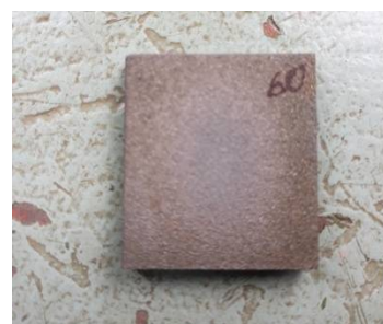
Fig 4.5 Erosion Test at 60°
