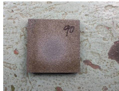
Fig 4.6 Erosion Test at 90°
