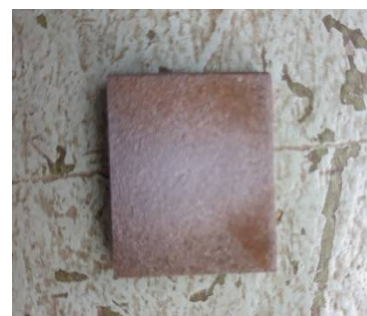
Fig 3.5 Erosion Test at 30°
