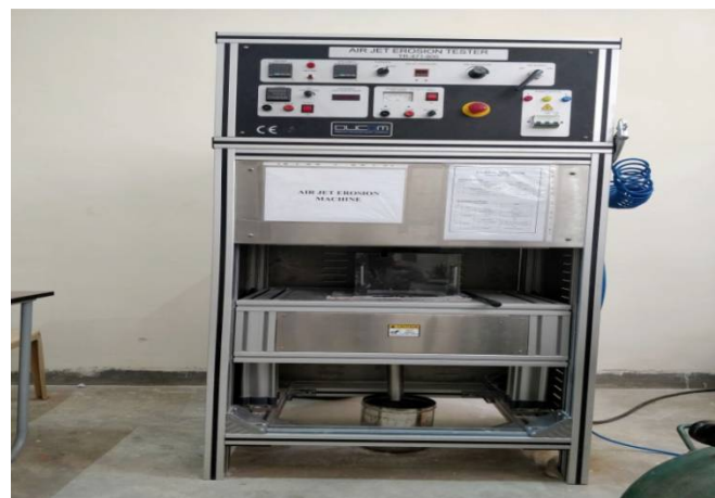
Fig 4.2 Air Jet Erosion Test Machine
