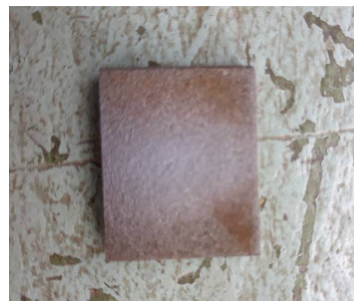
Fig 4.5 Erosion Test at 30°
