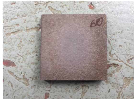
Fig 4.6 Erosion Test at 60°
