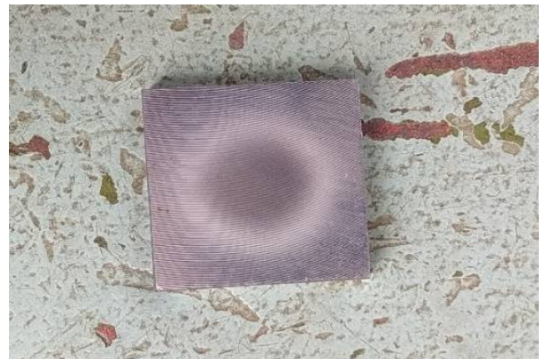
Fig 4.4 Erosion Test for 90°
