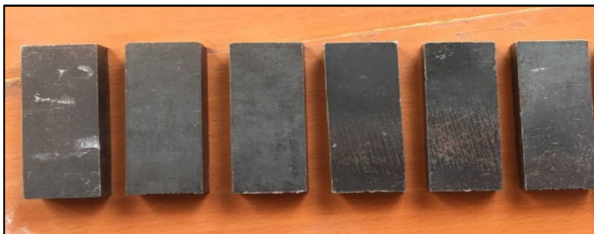
Figure 1 Standard test specimens of size 265×125×12mm
