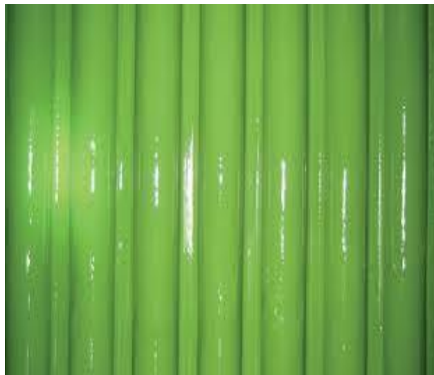
Fig. 3.4 Electro deposited inter metallic coatings
