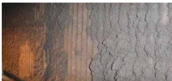
Fig. 2.4. Slag formed around boiler tubes
