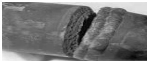
Fig. 2.7 Dissimilar metal weld failure
