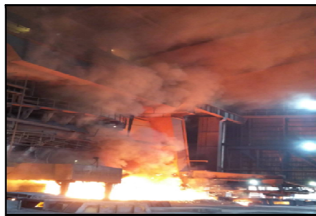
Fig-3.1: Tap closing failure caused disaster in cast house
