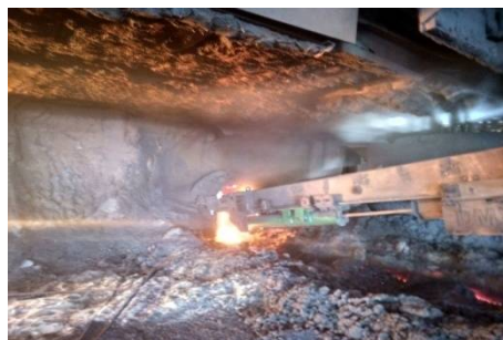
Fig-4.4(b) Tap hole closing using EMG system
