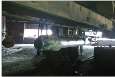
Fig-4.3: Fabricated Emergency mudgun fixed to drill machine guide frame
