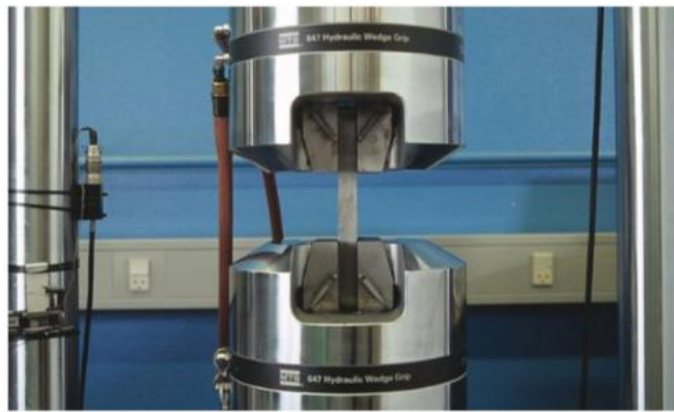
Fig 2.2 Loading arrangement of specimen for tensile strength test
