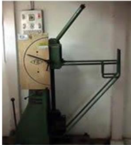
Fig 2.4 Experimental setup for impact test
