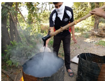
Figure : Keep mixing the melting plastic
