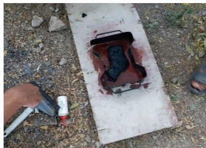
Fig: Press the mix tightly into the moulds. Air gaps will reduce the quality of your finished tile.
