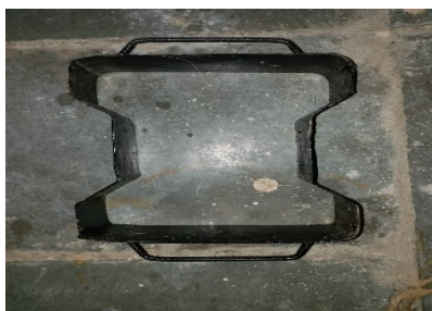
Figure : Check The Tile Moulds Are Clean And Oiled Before You Start Work.
