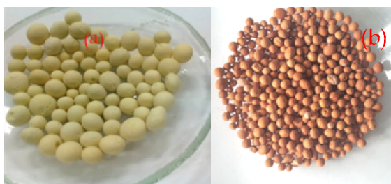
Fig. 4 Photo of \text{Al}_2\text{O}_3 pellets (a), and KI-impregnated pellets (b)
