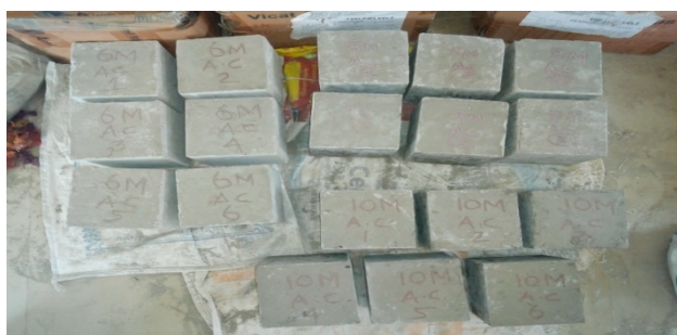
Fig3.1 Casting of GPC specimens
