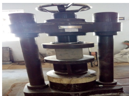
Fig4.1 Compressive Strength test for GPC Cubes
