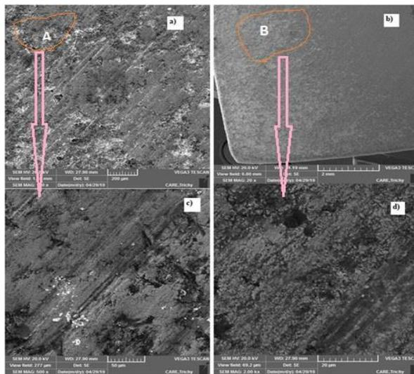
Fig.3 Images of the surfaces after wear test of (a) uncoated specimen (b) coated specimen (c) Enlarged view of portion of uncoated specimen (d) Enlarged view of portion of coated specimen
