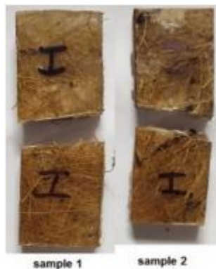
Fig.4: Impact test specimen
