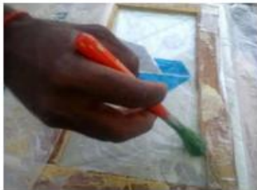
Fig.1 (a): Applying release gel
