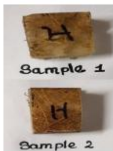
Fig.4: Hardness test specimen
