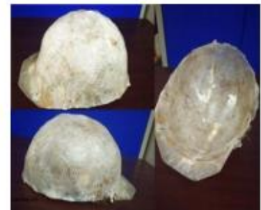
Fig.6: Fabricated helmet shell
