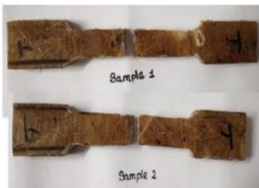
Fig.5: Tensile test specimen
