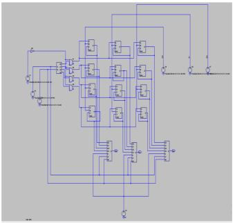
The above diagram shows that the RAM memory is designed using reversible logic. By using this technique, the D-flip flop can be replaced by fredkin gate.
