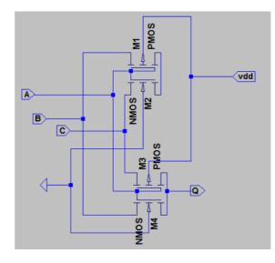
The above diagram shows the Fredkin gate, which is one of the reversible logic gates. It is the equivalent gate for D-flip flop. The existing method contains more transistors because of the usage of CMOS logic whereas in case of using reversible logic the transistor count can be reduced.
