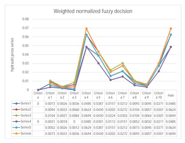
We studied the weighted normalised fuzzy decision matrix for the vertical and horizontal hydraulic press for the squeezing and flaring operations from that calculate the maximum value shown in the table as well as graph.
