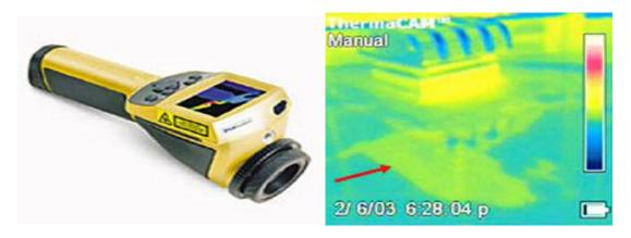
Figure 10. FLIR ThermaCAM ES IR camera and IR photo
