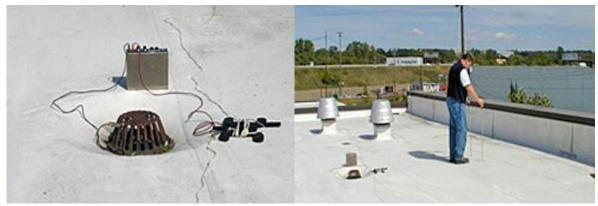
Figure 2. Low voltage test equipment
