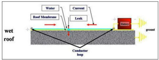
Figure 1: Low voltage electrical circuit
