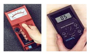
Figure 9. Tramex Capacitance meters
