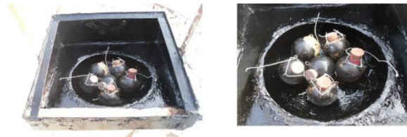
Fig. 3. Pictographic view of PC solar still model for experimental work.
