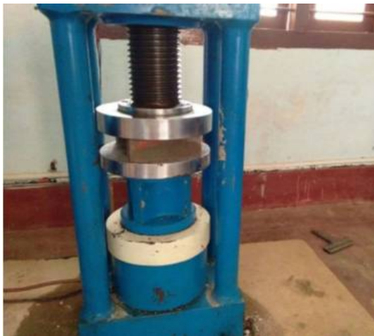
(a) Testing of compressive strength of paver block
