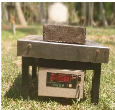
a) Weight of dry paver block
