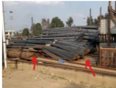
Fig 3: Oxidised safety stock.
