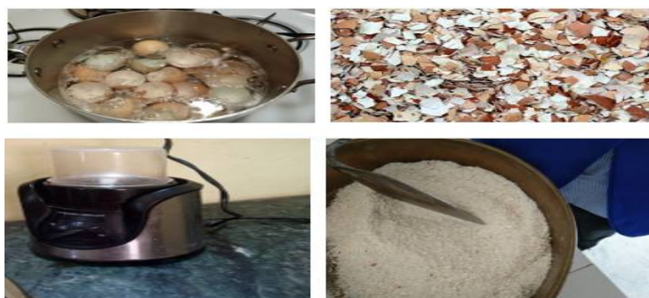
Fig 5 Processing of egg shell waste (i) washing (ii) air drying (iii) grinding (iv) sieving
