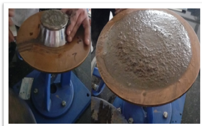
Plate 1: Flow Table Test
