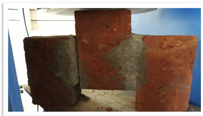
Plate 2: Triplet Shear Bond Strength Test Set-up
