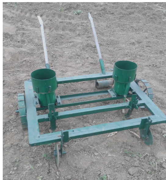
Fig. 6. Photograph of the fabricated conservation planter
