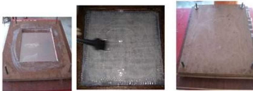
Figure 1: Hand Layup technique
