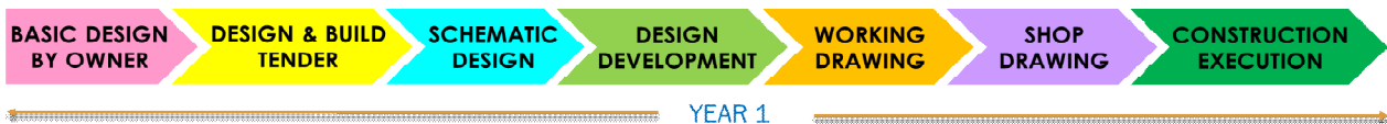
Fig IV.1: Comparison of flow/ stages of DED implementation with design and build implementation
