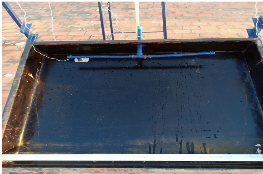
Figure 3.3 a Flat absorber
