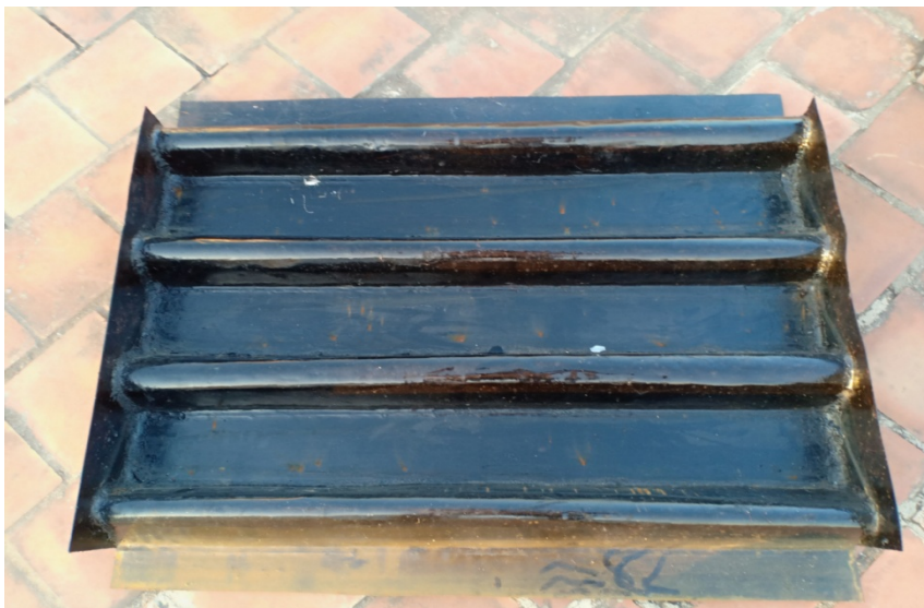
Figure 3.3 b Steeped absorber with grooves
