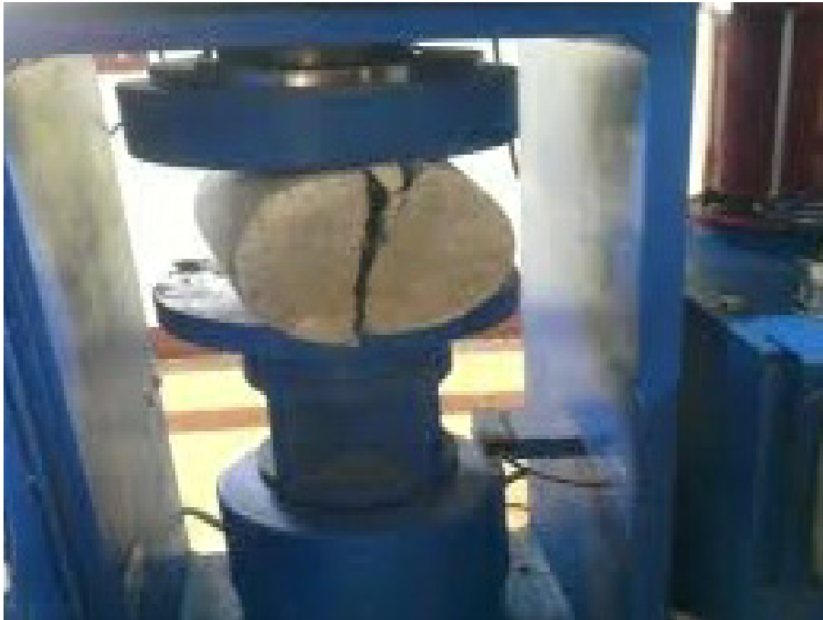
Fig 6.3.3 Split tensile testing of cylinder
