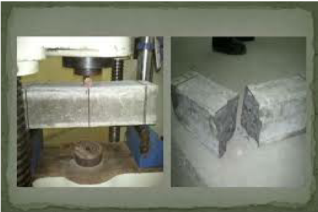
Fig 6.3.2 Testing of prism for flexural strength
