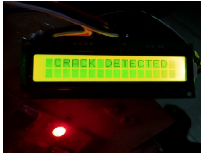
Fig. 3: LCD Displaying Crack Detected Message
