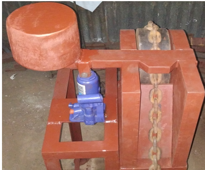
Fig (6.3): fabricated model of moveable hydraulic jockey
