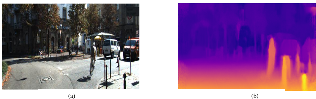
Fig. 1. Depth map (brighter pixels are closer to camera) (a) Original image (b) Corresponding depth map.
