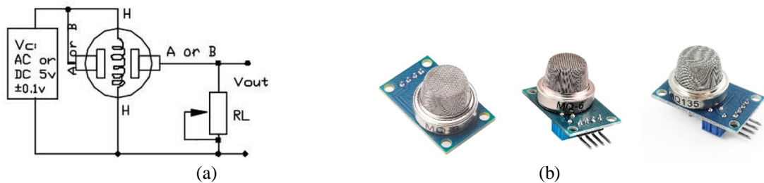
Fig. 4. (a) Internal circuit of an MQ gas sensor, (b) MQ gas sensor modules
