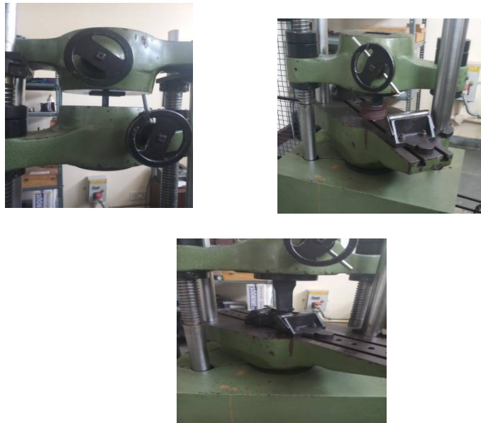
Fig 8: Tensile Test (top left), Compression Test (top right) and bending test (below)
