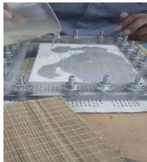
Fig 7: Hand lay-up process
