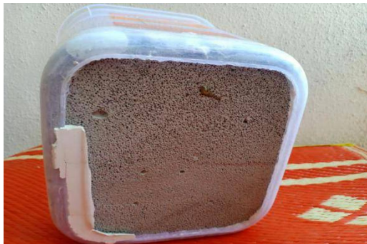
Fig no 5.6 Porous concrete (bottom view)
