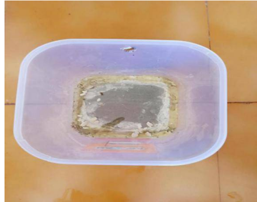
Fig no 5.5 Porous concrete fixed in bottom of container
