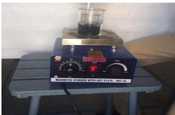
Figure 4 (a) Mixing of acetone with CNTs
