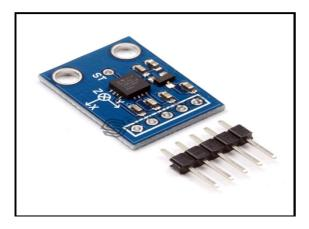
VIBRATION SENSOR ADXL335: Vibration sensors are used to measure displacement, proximity, linear velocity and acceleration. Here in this project we are using vibration sensor which detect the seismic vibration of earth. The
