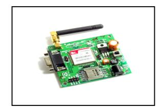
The SIM900 is a complete Quad-band GSM/GPRS solution in a SMT module which can be embedded in the customer applications. Featuring an industry-standard interface, the SIM900 delivers GSM/GPRS 850/900/1800/1900MHz performance for voice, SMS, Data, and Fax in a small form factor but we use only SMS alert. The communication of GSM digitizes and reduces the data, then sends it down through a channel with two different streams of client data, each in its own particular time slot.
