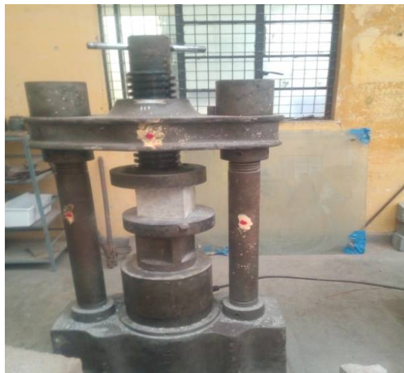
Fig.5.1. Compressive Strength Test
