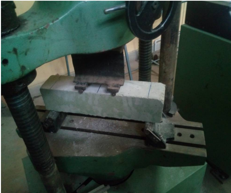
Fig.5.3. Flexural Strength Test
