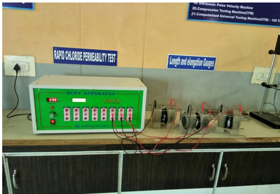
Fig.5.4. Test setup for RCPT test
