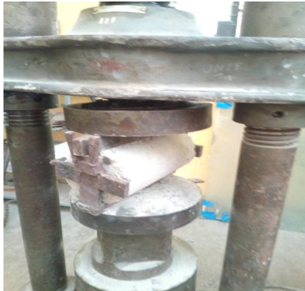
Fig.5.2. Split Tensile Strength Test
