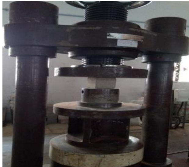
Fig 3.1 Compressive strength test for cement mortar cubes
