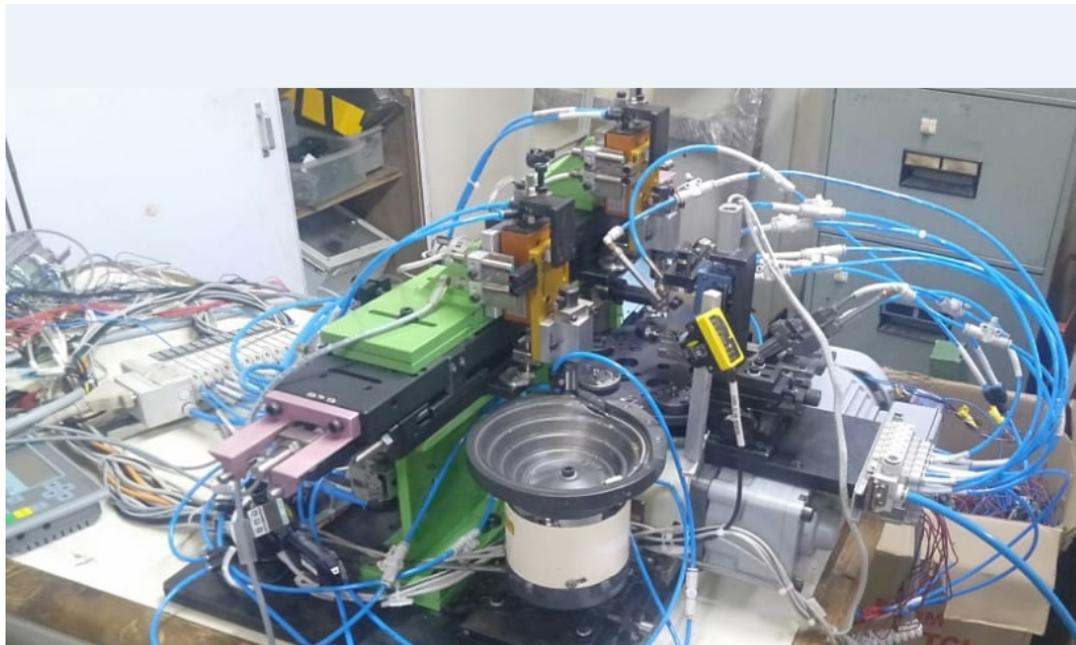
*Fig 3 OILING MACHINE FOR CANON PINION*
