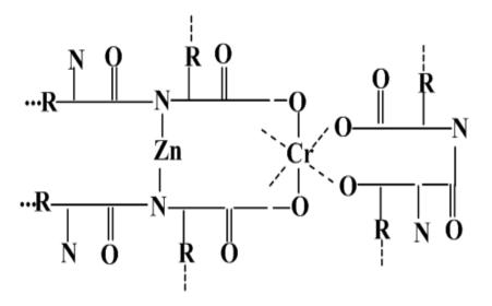
Fig. 1: Model of Zn-Cr combination tanning structure [24].
