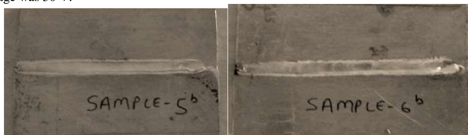
Fig -8 Both side MIG welded samples prepared with (a) welding current 180 A, welding speed 3 mm/s (b) welding current 180 A, welding speed 3.5 mm/s
