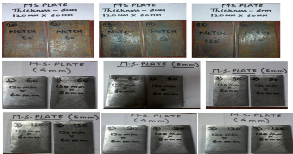
Fig. 6. Figure of M.S. plate of dimension 120mmX60mmX6mm
