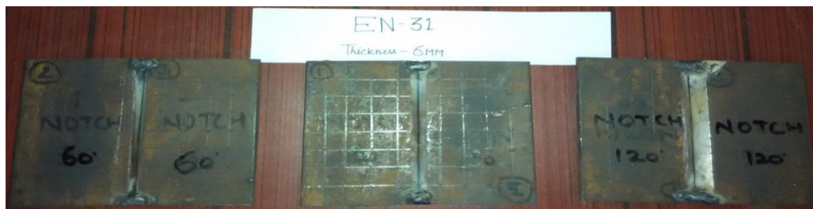
Fig. 9. Figure of EN-31 plate of dimension 120mmX60mmX6mm
