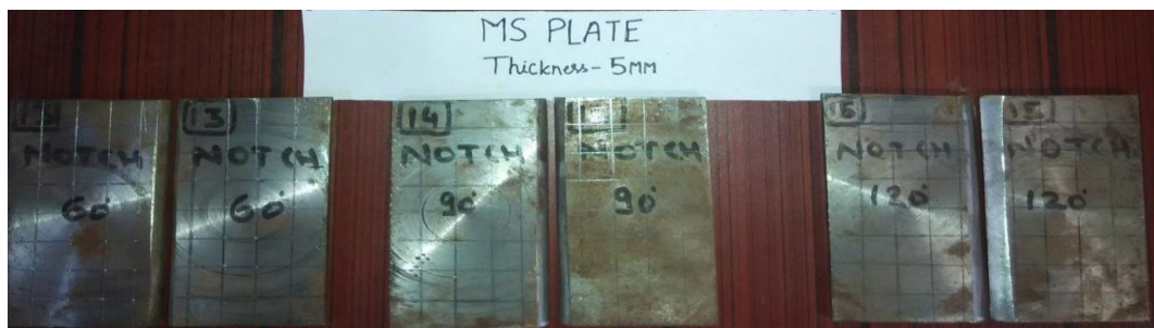
Fig. 7. Figure of M.S. plate of dimension 120mmX60mmX5mm
