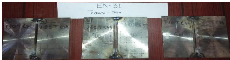
Fig. 10. Figure of EN-31 plate of dimension 120mmX60mmX5mm
