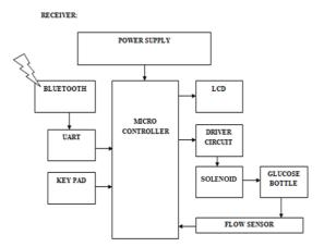
The circuit has a receiver and a transmitter. The controller in the receiver is connected to the Bluetooth through the UART. The Keypad and LCD module is also connected to the controller. The flow sensor and the driver circuit is connected to control the glucose flow in the glucose bottle using a solenoid value.
