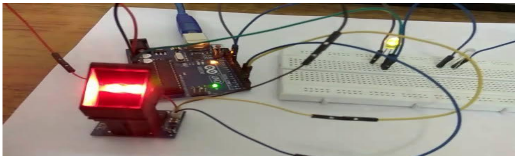
Fig. 5. Interfacing fingerprint with Arduino
