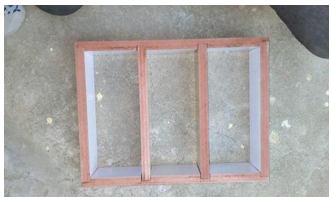
Fig 2 Mould for Paver blocks
