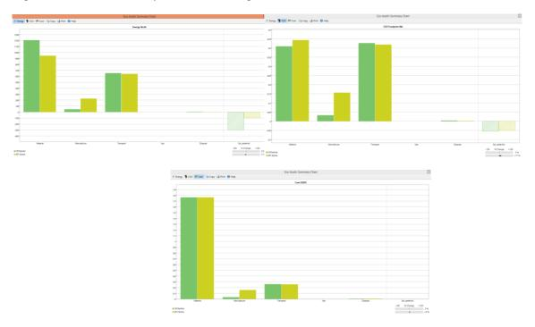
It can be concluded from the above charts that for materials and transport category, energy required for Tetra Pak is more than PET bottle and for manufacturing, energy required to produce PET bottle is more than Tetra Pak. Co<sub>2</sub> emitted during manufacturing and material production is more for PET bottle than Tetra Pak whereas Tetra Pak
