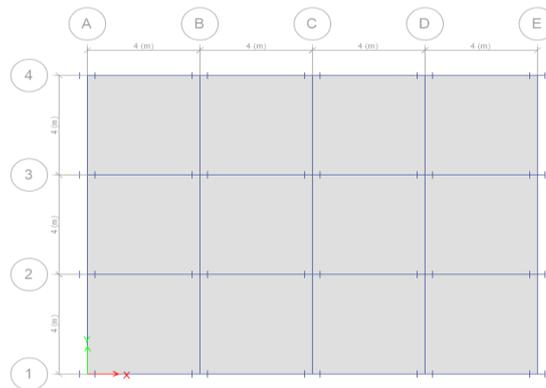
Fig.1.Floor Plan of Steel Frame Story
