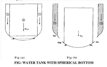
Alternatively, the downward load may be calculated from the weight of water and tank bottom of the part i.e. W2 less upward react ion of the support as shown in Fig. For section which cuts the tank bottom inside the support, the reaction has to be considered with the weight of water and tank of the annular part.
