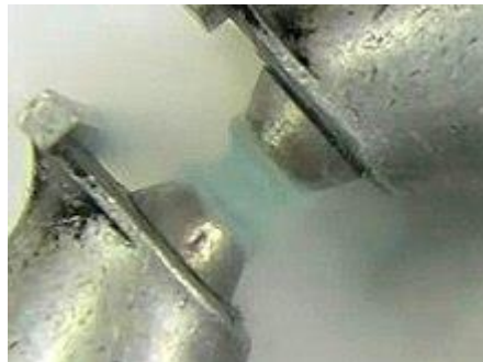
When liquid oxygen is poured from a beaker into a strong magnet, the oxygen is temporarily suspended between the magnet poles, owing to its paramagnetism.
