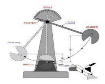
The process of evaluating the toughness, impact strength and notch sensitivity of engineering materials .This type of test is considered to be called as impact test.
