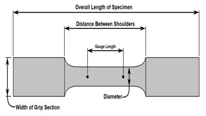
Tensile testing also known as tension testing is a fundamental materials science and engineering test in which is subjected to a controller tension until failure. It's a destructive test process that provides information about the tensile strength yield strength and ductility of the metallic material.
