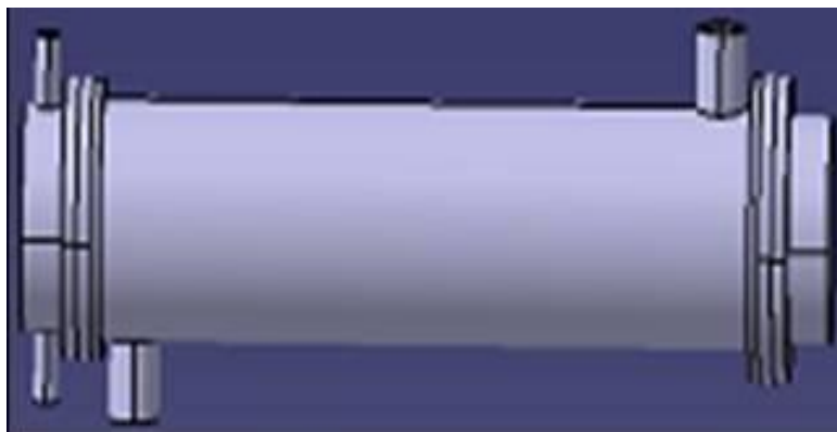
Fig8: Fully Assembled Heat Exchanger
